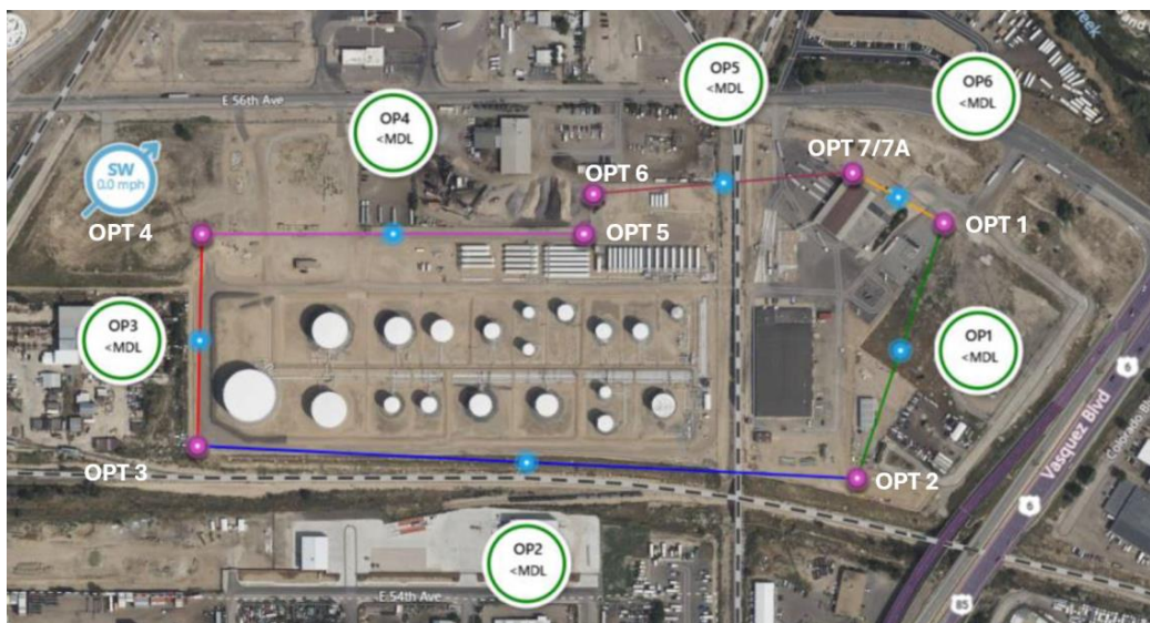
Figure 3-1. Approximate Layout of the Open-Path Analyzers, Retroreflector Locations, and Meteorological Station
