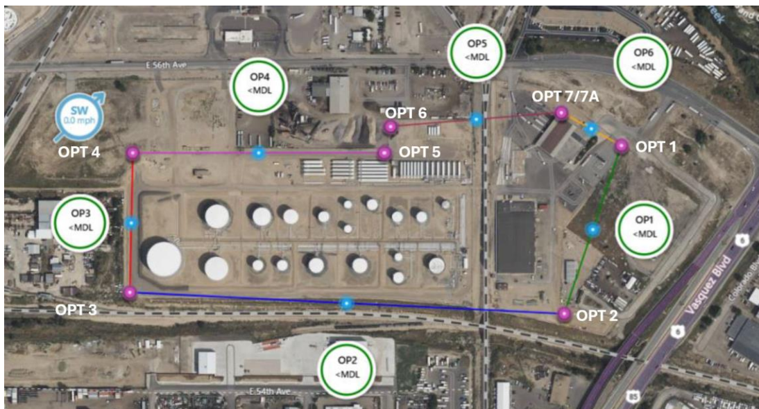
Figure 5-1. Location of Point Samplers/Monitors Should Any Fenceline Equipment Become Non-Operational. The blue circles correspond to the location of the passive tube samplers.
